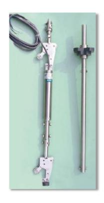
However, for large number of sensors in a single string, routing of individual sensor cable to the top is a cumbersome, costlier affair. It limits the number of sensors to be used in a single borehole and also increases the weight of the IPI assembly.
