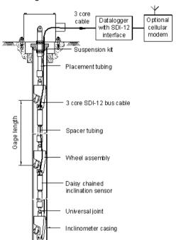
EAN-52M In-place inclinometer system with SDI-12 bus interface to SDI-12 compatible datalogger
