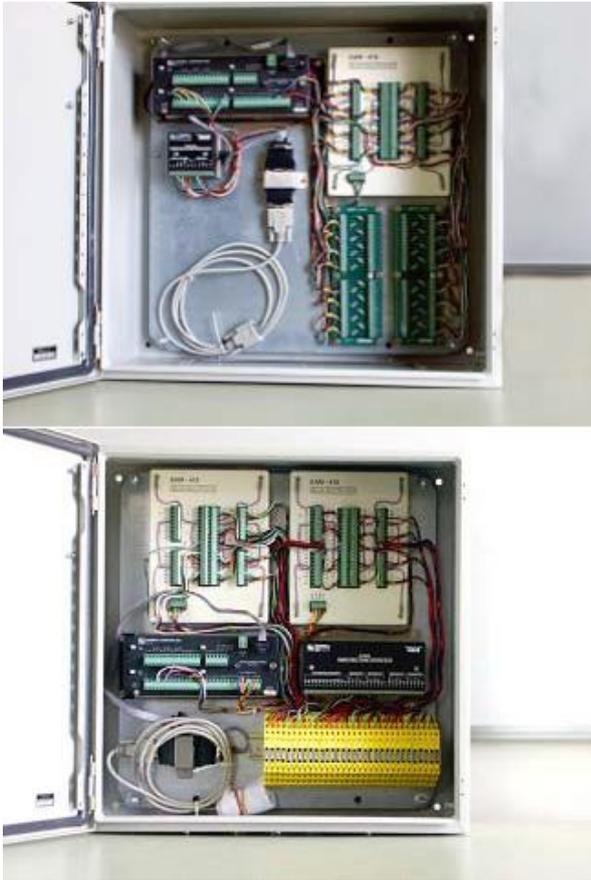
EDAS-10's digital output ports in combination with suitable device drivers can interface with many commercially available control devices like valve actuators, motors, solenoids, relays, etc. They can also be used to control external alarm annunciators like lamps and buzzers.
