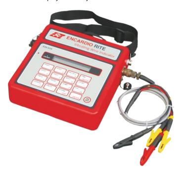
Model EDI-51V indicator can store calibration coefficients of maximum 500 number of sensors. It has capacity to store either 4500 readings from any one sensor or about 9 sets of readings from all 500 sensors. Each reading is stamped with date and time at which the measurement was taken.
